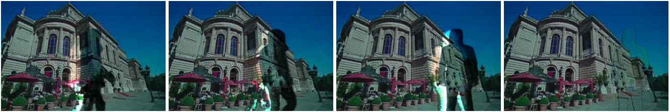
Figure 1: Luminance correction for dynamic change of luminance properties with a people cut across in front of the projected wall. The correction was dynamically applied according to his movement, and finally in the right edge image, he stopped and completely disappeared.
